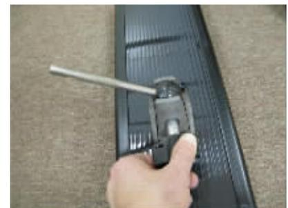
Figure 4b – The “bar handle” version of the MAM for the CL-255P/PMD and the CL-455P/PMD
