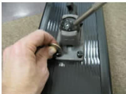
**Figure 5a – Unlocking / locking the MAM screws with a coin**
