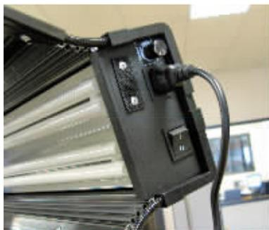
**Figure 12 – Power plug, power switch (and dimmer on CL-255PMD only)**
