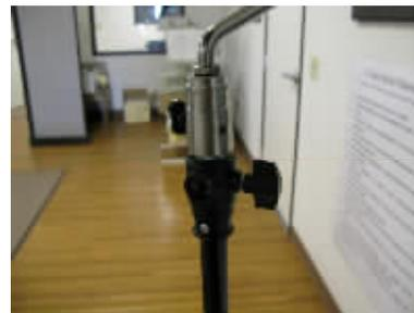
**Figure 11 – CL-MPSA baby adapter attached to baby stand**
