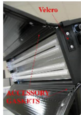
**Figure 13 – Accessory gaskets and Velcro attachments**
