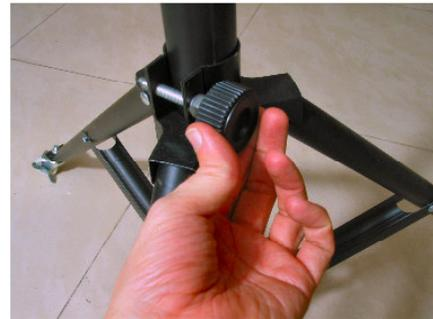
Figure 3 - Tighten bottom extension knob
