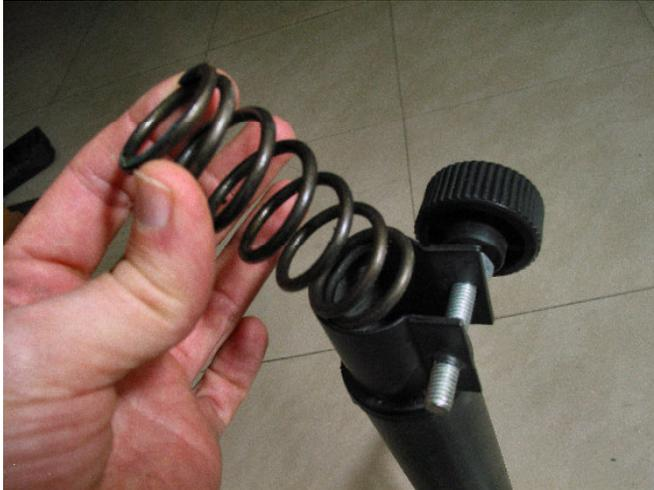
Figure 4 - Insert spring into stand
