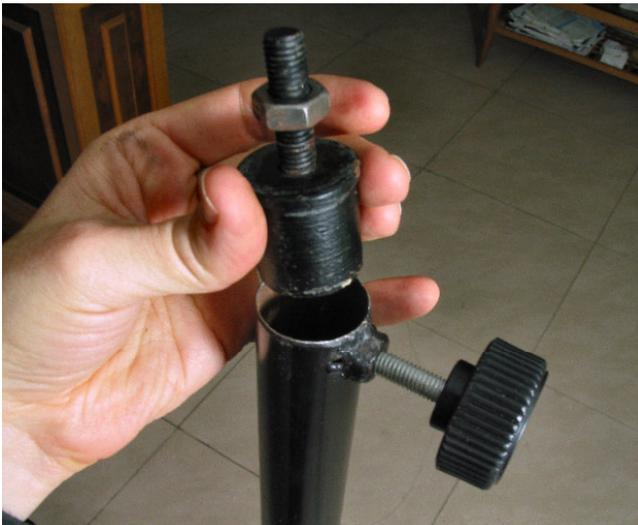
**Figure 7 - Inserting stand to yoke adapter**
