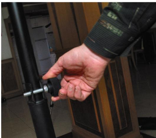
Figure 6 - Tighten extension knob
