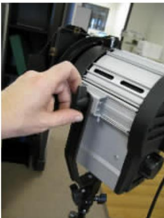
**Figure 11 – Angle adjustment thumbscrew.**
