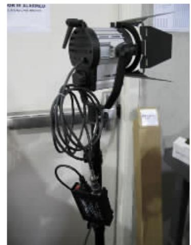
**Figure 7 – Ballast attached to stand with carabiner**
