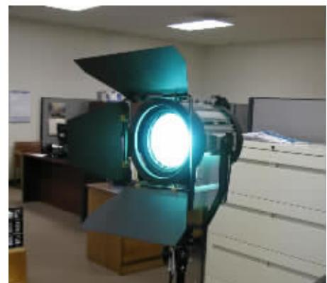
**Figure 8 – The bulb takes up to five minutes to stabilize color temperature.**
