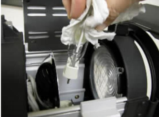
**Figure 4 – Inserting the bulb**
