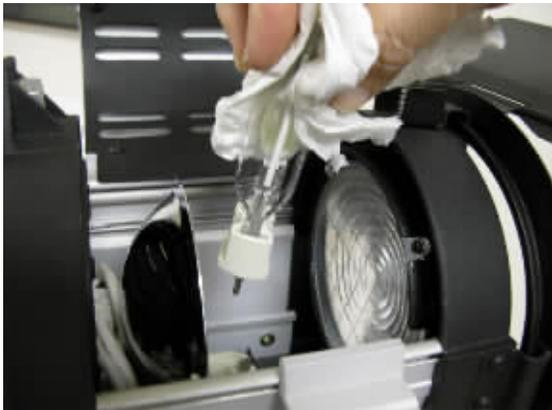
**Figure 4 – Inserting the bulb**
