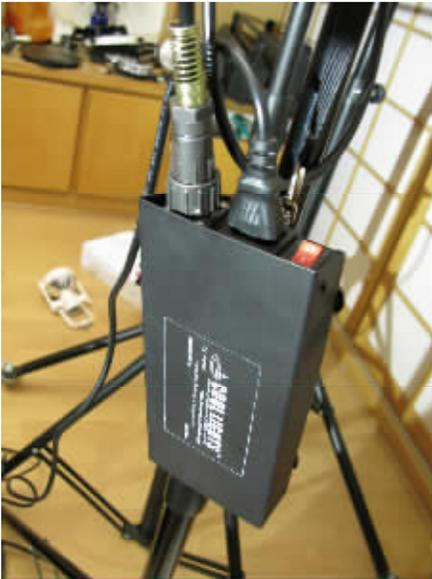
**Figure 6 – The connectors and switch on the ballast**
